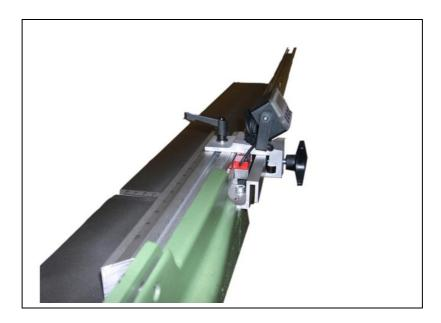
The beam is fitted onto the extension table by means of the screws in the same way as the standard beam is fitted.
