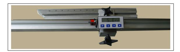
The stop beam is fitted into the stop block with the digital display.
