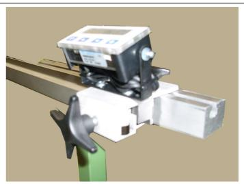
The digital display is pushed into the beam from the end – as shown on the pictures.
